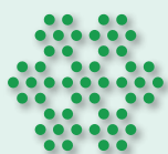
Rope 6 × 7 + WC for Webnet rope Ø 1.0 mm, 1.5 mm, and 2.0 mm
