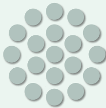
↑ Inox-Litze Toron Inox Stainless steel strand 1 x 19 E = 1,4 - 1,7 · 10 5 N/mm 2
